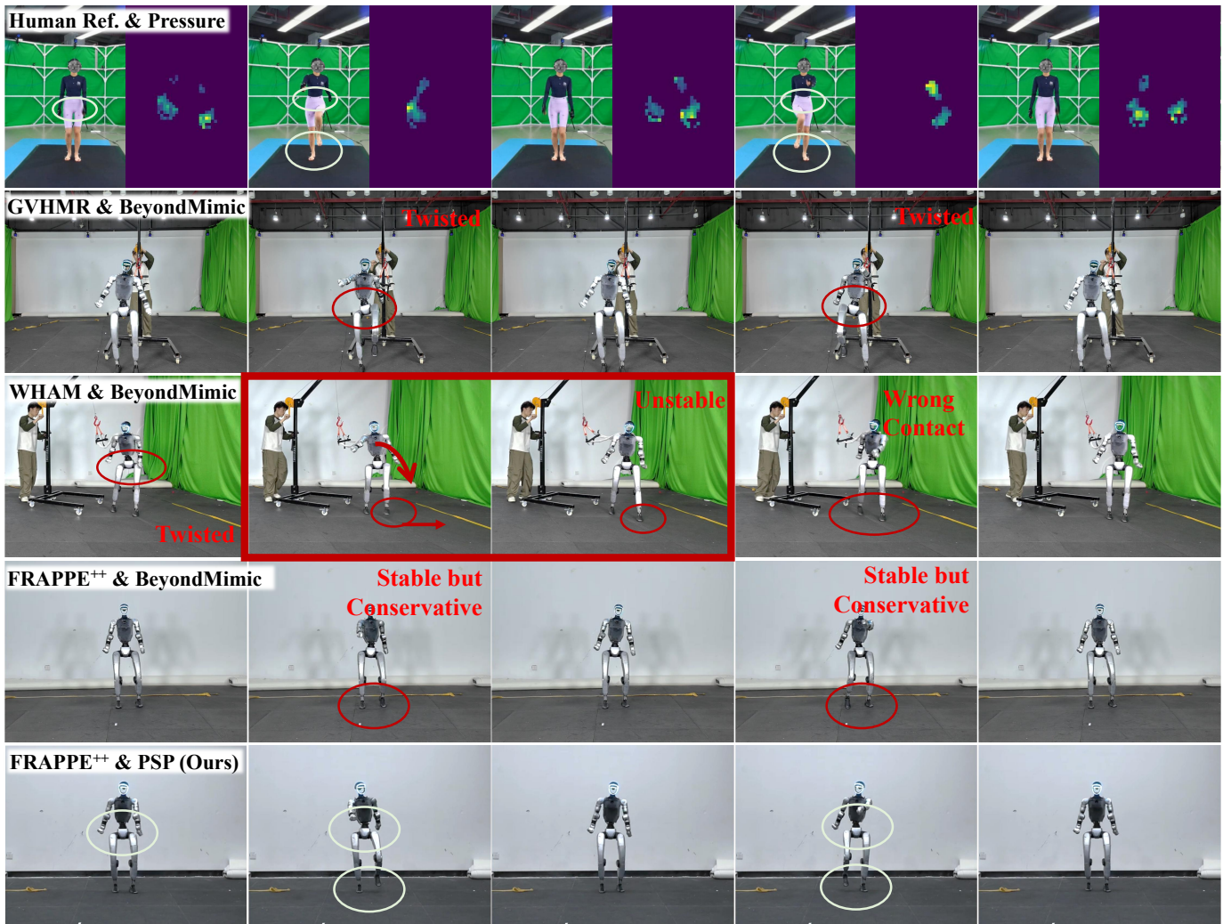
Fig. 8. Real-world humanoid motion imitation results. Rows show execution results under different reference sources and control policies. Low-quality references (GVHMR, WHAM) lead to twisted postures and instability, while FRAPPE ++ with BeyondMimic achieves stable but conservative foot placement. FRAPPE ++ with PSP (Ours) produces stable execution with more natural foot contact dynamics (white circles), validating sim-to-real transfer of pressure supervision.
